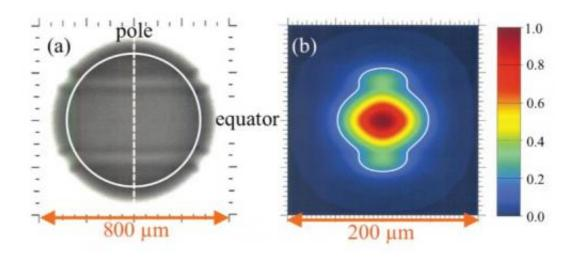
Simulated backlit (a) and core emission (b) images showing a feature that approximates the effect of a 45-nanometer tent.
