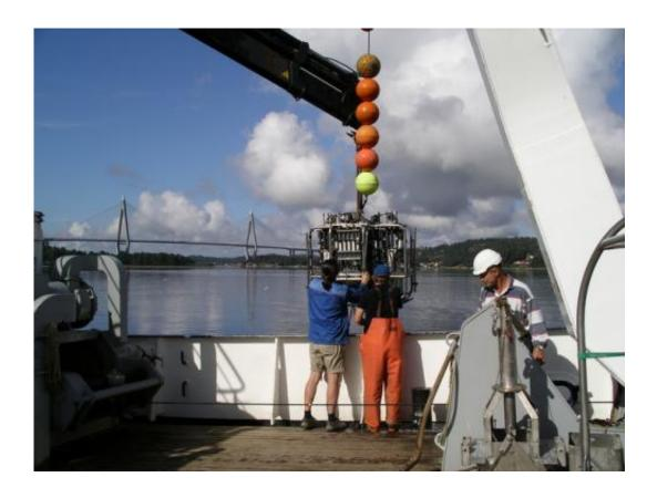
Deployment of scientific equipment to determine the water quality in the Byfjord.
