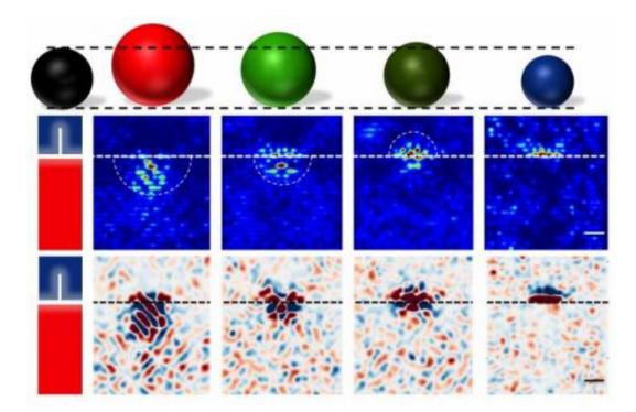
Simulations show the effects of dislocations in cerium dioxide on the redistribution of differently sized dopant atoms, replacing a cerium atom in the crystal lattice. The results reveal different amounts of segregation around the dislocation caused by the differently sized elements. The sizes of the other atoms are compared to a cesium atom (left, in black). The white dashed line shows the plane of the dislocation caused by strain.
