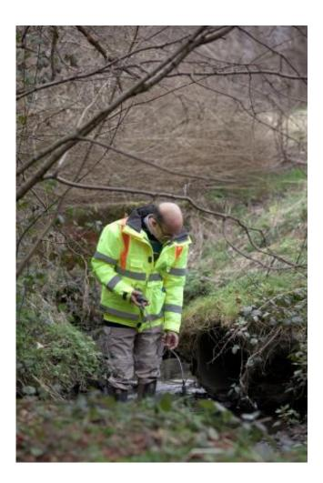
Professor Lerner is testing for sewage pollution in a stream in Sheffield, UK, using a conductivity and temperature meter -- a more expensive but less effective method than using tampons and UV lighting. Credit: University of Sheffield
