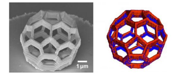
3D image of the buckyball structure investigated. In the right picture the distribution of Cobalt is shown in orange. (The solid line corresponds to 1 micrometre or 1 thousandth of a millimetre).
