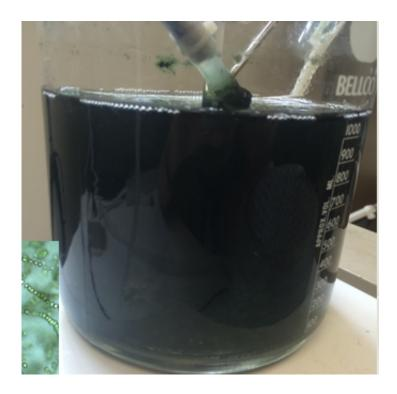
Researchers have been experimenting with methods of growing cyanobacteria colonies in photobioreactors on a large scale with the goal of licensing the technology to an agricultural company. Credit: Penn State
