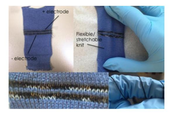
Using industrial knitting machines in the Shima Seiki Haute Technology Laboratory, Drexel researchers are searching for the best capacitive yarn to use in energy storage textiles.
