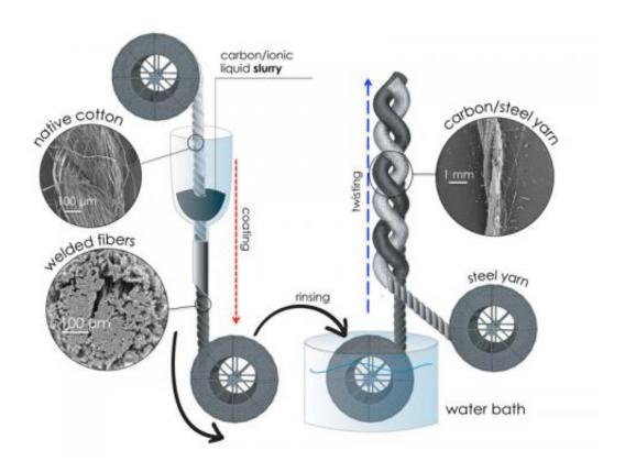
Drexel researchers have developed an effective process for coating yarn with activated carbon and twisting it with stainless steel to make it capacitive.
