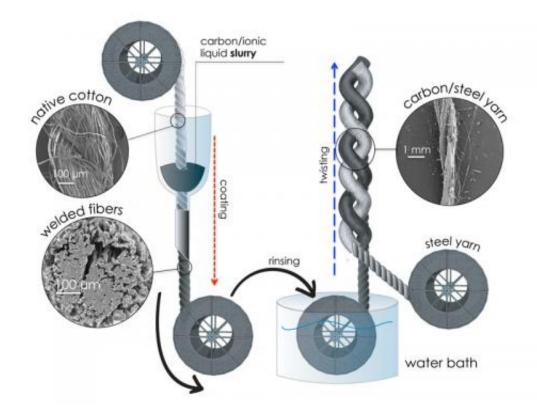
Drexel researchers have developed an effective process for coating yarn with activated carbon and twisting it with stainless steel to make it capacitive.
