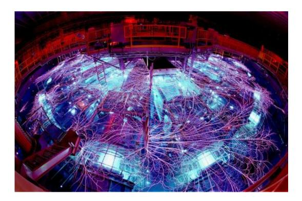
The Z machine is in Albuquerque, N.M., and is part of the Pulsed Power Program, which started at Sandia National Laboratories in the 1960s. Pulsed power concentrates electrical energy and turns it into short pulses of enormous power, which are then used to generate X-rays and gamma rays. Credit: Randy Montoya
