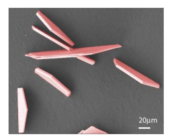
By adjusting the fabrication technique, researchers can make different semiconductor structures, including nanoplates that lie flat or stand upright. Credit: Koski lab / Brown University
