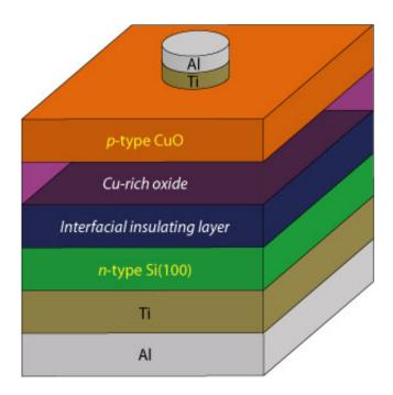
High-performance solar cells can be produced using inexpensive materials by minimizing the copper-rich and interfacial insulating layers in the interface between the cupric oxide (CuO) and silicon (Si) layers. Credit: A\*STAR Institute of Materials Research and Engineering
