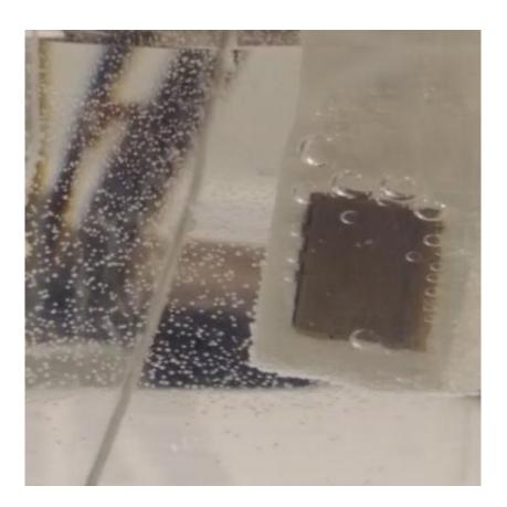
Water splitting into hydrogen on a metal wire and oxygen on the catalyst.
