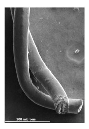
Pairs of carbon nanotube fibers have been tested for potential use as implantable electrodes to treat patients with neurological disorders like Parkinson's disease. The fibers invented at Rice University proved to be far better than metallic wires now used to stimulate neurons in the brain. Credit: Pasquali Lab/Rice University
