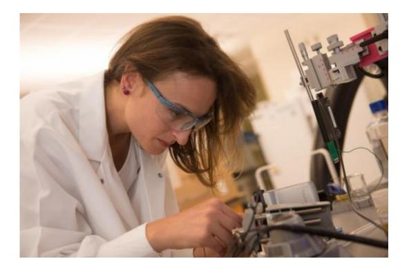
Flavia Vitale, a postdoctoral researcher at Rice, prepares carbon nanotube fibers for testing. Vitale is lead author of a new study that determined the thread-like fibers made of millions of carbon nanotubes may be suitable as electrodes to stimulate the brains of patients with neurological diseases. Credit: Jeff Fitlow/Rice University
