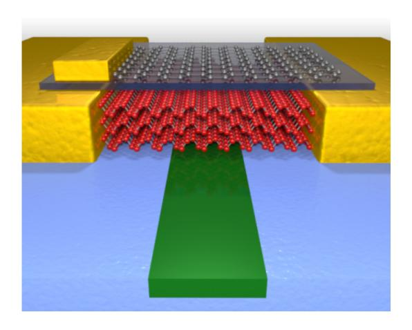
This illustration shows the high performance photodetector which uses few layer black phosphorus (red atoms) to sense light in the waveguide (green material). Graphene (gray atoms) is also used to tune the performance. Credit: University of Minnesota, College of Science and Engineering
