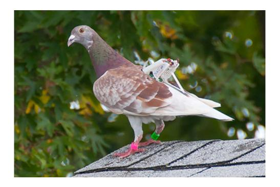
The image shows a prototype for a bio-data collector for birds, which relies on a pendulum that resonates with a bird's wing-beat frequency to generate electricity. The prototype was tested on trained pigeons that would return the device. Credit: Michael Shafer
