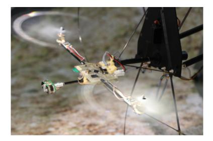
The BeeRotor robot, equipped with an eye inspired by that of insects. Credit: Expert & Ruffier (ISM, CNRS/AMU)
