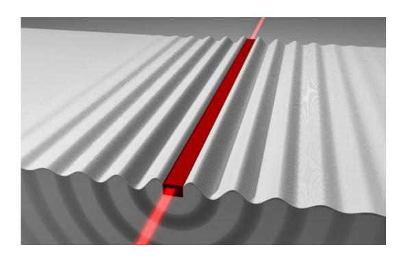
This illustration shows the emission of phonons (sound waves) from a nanometer scale waveguide, as optical waves flow through it. Credit: Yale University
