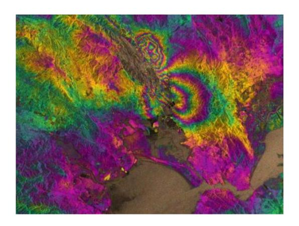
Satellite radar image of the magnitude 6.0 South Napa earthquake. The "fringe" rainbow pattern appears where the earthquake deformed the ground's surface, with one full cycle of the color spectrum (magenta to magenta) showing 3 centimeters of change. Satellite data like this can now be used to give researchers an understanding of an earthquake and its impacts within days. Credit: the European Space Agency.
