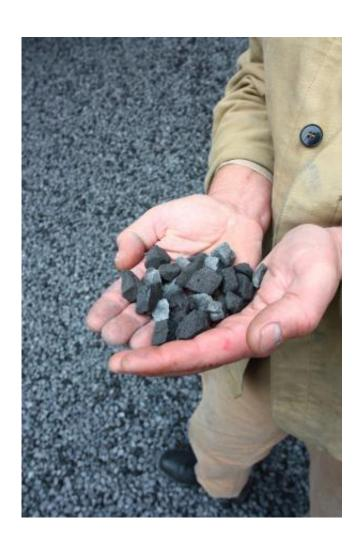
Processed material recovered from slag. Credit: Fraunhofer UMSICHT
