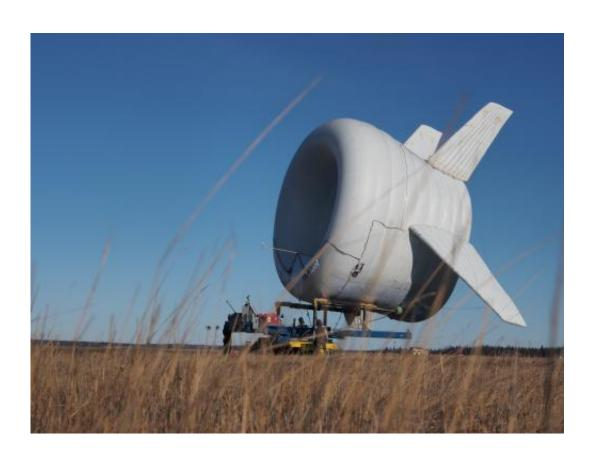
Much like other tethered balloons, the Altaeros BAT can lift communication, Internet and sensory equipment alongside the turbine to provide additional services for customers. The addition of payload equipment does not affect its
