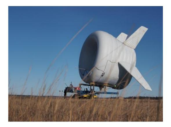
Much like other tethered balloons, the Altaeros BAT can lift communication, Internet and sensory equipment alongside the turbine to provide additional services for customers. The addition of payload equipment does not affect its
