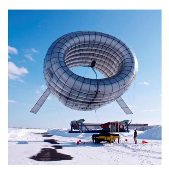
Most wind turbine manufacturers are competing to build taller turbines to harness more powerful winds above 500 feet, or 150 meters. Altaeros is going much higher with their novel Buoyant Airborne Turbine: the BAT. The Altaeros BAT can reach 2,000 feet, or 600 meters. Credit: Altaeros Energies
