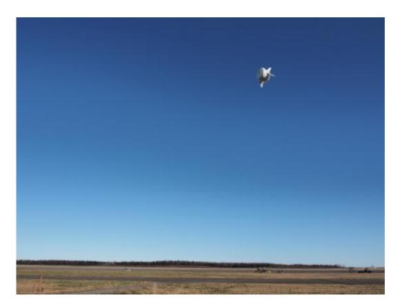
The key enabling technologies include a novel aerodynamic design, custommade composite materials, and an innovative control system. The heliuminflatable shell channels wind through a lightweight wind turbine, self-stabilizes, and produces aerodynamic lift, in addition to buoyancy. Multiple high strength tethers hold the BAT in place and a single conductive tether transmits power to a mobile ground station. Credit: Altaeros Energies
