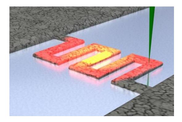
Artist's conception of plasmon energy expansion thermometry showing a focused electron beam penetrating a 100 nanometer wide aluminum wire atop a thin glass window. The wire's temperature is mapped by scanning the electron beam. Credit: CEMMA and Regan Group
