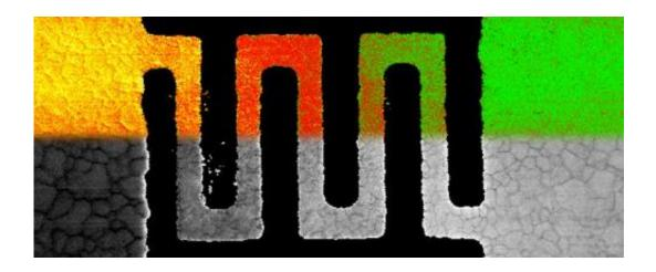
This composite image shows density (grey) and temperature (color) maps of a 100 nm-wide polycrystalline aluminum wire. The temperature is computed from the density using aluminum's known thermal expansion. Lower densities appear at crystal-grain boundaries, which are atomic-scale features, and where thermal expansion has caused the aluminum to expand. One end of the wire (green) is near room temperature, and the other (orange) is 160 K warmer. Credit: USC CEMMA & UCLA Regan Group
