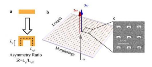
Metamaterial arrays whose geometry varied gradually from a symmetric bar to an asymmetric U-shape were used to compare the predictive abilities of Miller's rule and a non-linear light scattering theory. Credit: Xiang Zhang, Berkeley Lab
