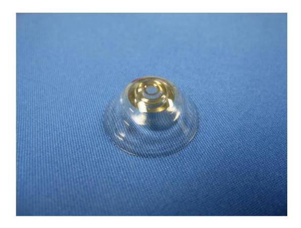
A close-up view of the latest prototype of the telescopic contact lens. Credit: Eric Tremblay and Joe Ford / EPFL.
