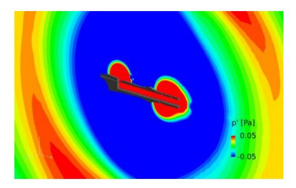
Contours of pressure fluctuation around recorder with opened tone holes. Credit: Toyohashi University of Technology
