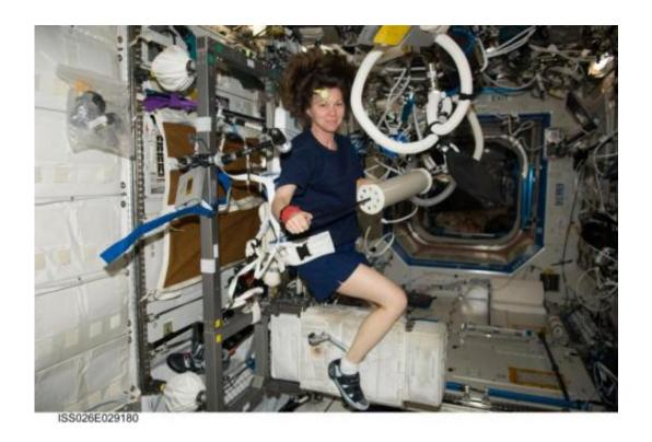
Catherine (Cady) Coleman, Expedition 26 flight engineer, performs calibrations on the VO2max Portable Pulmonary Function System (PPFS). The PPFS is located next to the Cycle Ergometer with Vibration Isolation System (CEVIS) so astronauts can measure their oxygen consumption while riding the CEVIS. Credit: NASA
