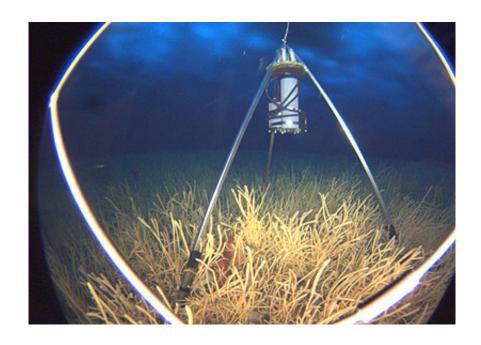
SeeStar camera system mounted on a tripod beneath the Antarctic ice near McMurdo Station. Credit: Stacey Kim, Moss Landing Marine Laboratories.
