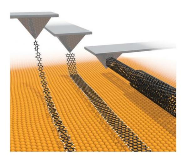
Researchers investigated the superlow friction of the chain structures above. They found that superlubricity can theoretically hold for tens of cemtimeters and disappears above a critical chain length, which depends on a material's intrinsic properties. Credit: Ma, et al. ©2015 American Physical Society
