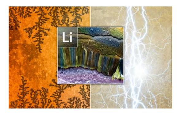
Large-scale use of high-energy rechargeable lithium metal batteries is limited by harmful deposits called lithium dendrites. A recent JCESR study evaluated the effect of an electrolyte additive that suppresses lithium dendrite formation.
