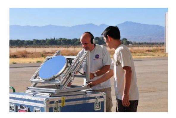
Principal Investigator Haris Riris (left) and Stewart Wu prepare a prototype of the methane sounder (the mirror is an alignment tool) before demonstrating it aboard NASA's DC-8 research aircraft in 2011. Another flight is scheduled for later this year. Credit: Emily Schaller
