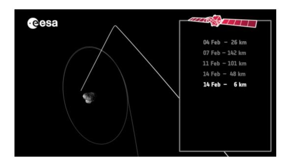
The relative position of Rosetta with Comet 67P/Churyumov–Gerasimenko at the moment of closest approach on 14 February 2015, when the spacecraft is just 6 km above the comet's large lobe. Credit: ESA/C. Carreau
