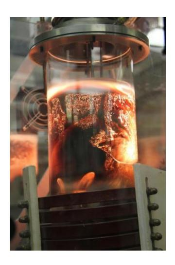
Scientists at the Critical Materials Institute, headquartered at the US Department of Energy's Ames Laboratory, have developed a new two-step process to make recycling rare-earth metals easier and more cost-effective. Here, magnesium is melted with magnet scrap in an induction furnace. Credit: US Dept. of Energy's Ames Laboratory
