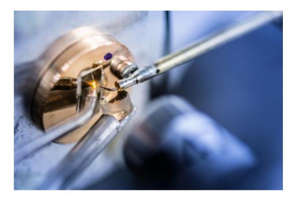
In order to generate oscillating polarisation, the researchers bend the laser with a nail (left). Thus, the active material is no longer symmetrical and becomes birefringent. Generally speaking, the more strongly a laser is bent, the faster the oscillation. Credit: RUBIN, photo: Schirdewahn
