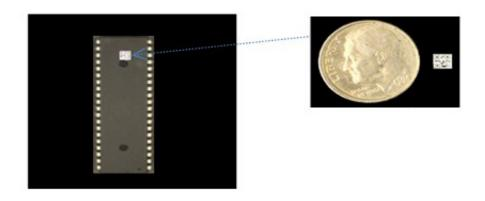
A 3.15 mm QR code storing an encrypted and compressed image shown placed on an integrated circuit and an image of the QR code placed next to a dime. Credit: Adam Markman/Brhram Javidi
