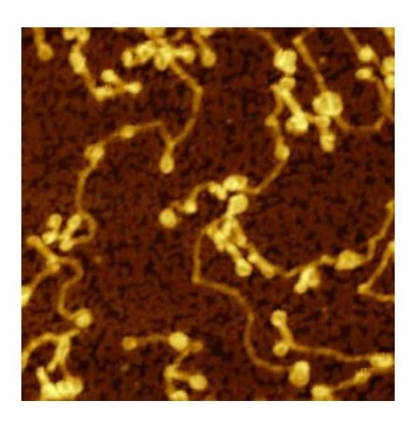
A detail of an atomic force microscopy image which shows amyloid fibrils of alpha-synuclein grown out of synthetic lipid vesicles. Credit: A.K. Buell
