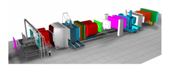
Artistic view of the 60 m long COMPASS two-stage spectrometer. The two dipole magnets are indicated in red.
