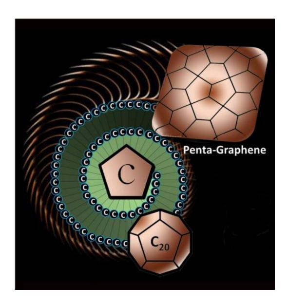
The newly discovered material, called penta-graphene, is a single layer of carbon pentagons that resembles the Cairo tiling, and that appears to be dynamically, thermally and mechanically stable. Credit: Virginia Commonwealth University
