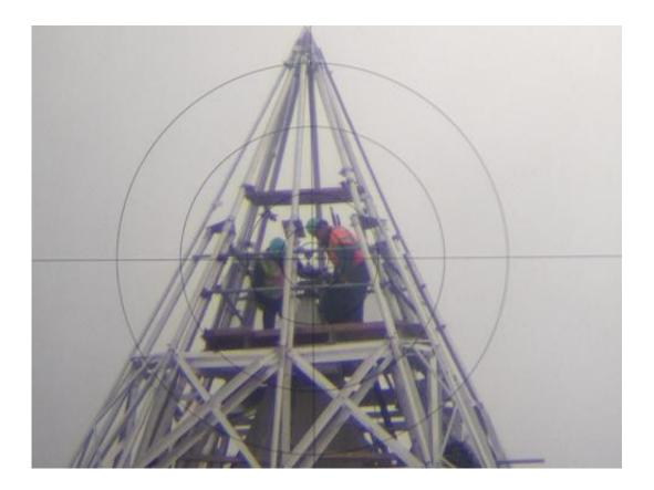
The view of the top of the Monument as viewed through the Total Station surveying tool, captured by placing a smartphone camera up to the eyepiece.
