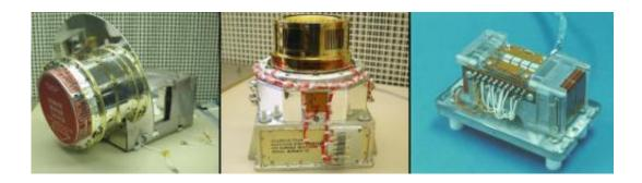
Three instruments will help measure the solar wind on the DSCOVR mission: (shown from left to right), the Faraday cup to monitor the speed and direction of positively-charged solar wind particles, the electron spectrometer to monitor electrons, and a magnetometer to measure magnetic fields. Credit: NASA/NOAA/DSCOVR
