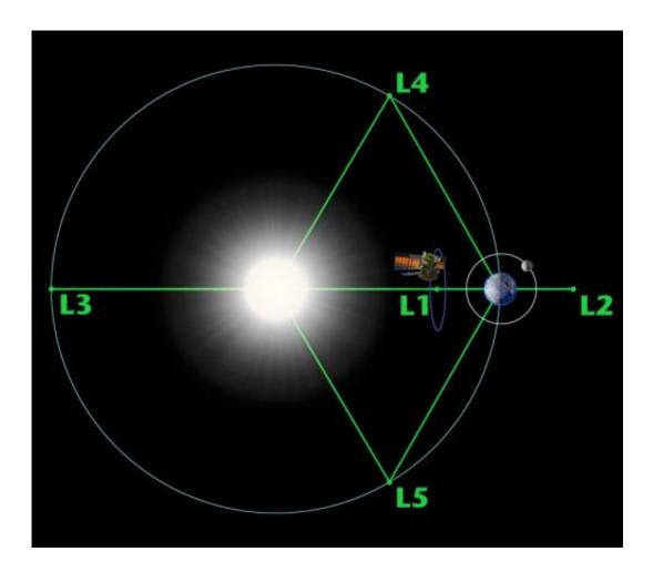
This is a diagram of the five Lagrange points associated with the sun-Earth system, showing DSCOVR orbiting the L-1 point. Image is not to scale. Credit: NASA/WMAP Science Team
