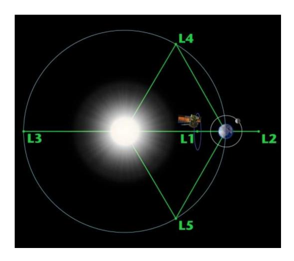
This is a diagram of the five Lagrange points associated with the sun-Earth system, showing DSCOVR orbiting the L-1 point. Image is not to scale. Credit: NASA/WMAP Science Team
