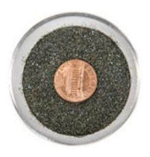
Oxygen carriers are similar in texture to sand. The oxygen carrier pictured here blends magnesium oxide and hematite.
