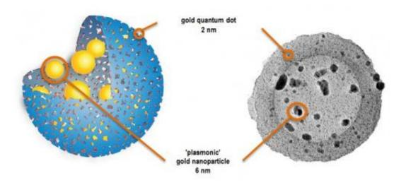
Diagram and electronic microscopy image of a "quantum rattle": a porous silica shell (in blue in the diagram) is filled with gold dots, all on a nanometric scale. Gold is present in two forms: particles smaller than 2 nm (dots) in the pores of the shell, and larger particles (7 nm) in the central cavity. Credit: Mathew Hembury, Ciro Chiappini Glenna L. Drisko et al, with the authorization of *PNAS* These images are available at the CNRS photo library, phototheque@cnrs.fr
