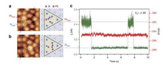
(a) and (b) show the two stable states created when two Pb and three Si atoms are rearranged in response to being scanned by the tip of a scanning tunneling microscope. The two states, which are chiral inversions of each other, correspond to a high-current state and a low-current state, allowing the cell to function as a new type of atomic-scale switch. Credit: Inami, et al. © 2015 Macmillan Publishers Limited
