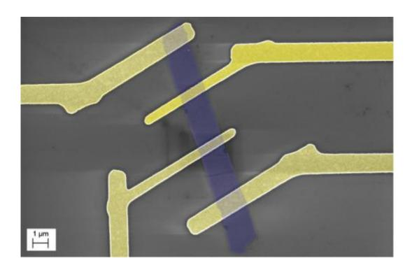
Atomic force microscopy image of a representative MoS2 thin-film transistor. Credit: Alexander A. Balandin/University of California-Riverside
