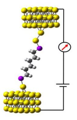
A single molecule of hexane (six carbon atoms) with sulfur atoms at each end, between two gold electrodes. A new technique invented at UC Davis allows better measurements of the properties of such circuits and could boost research in nanotechnology. Credit: Josh Hihath/UC Davis
