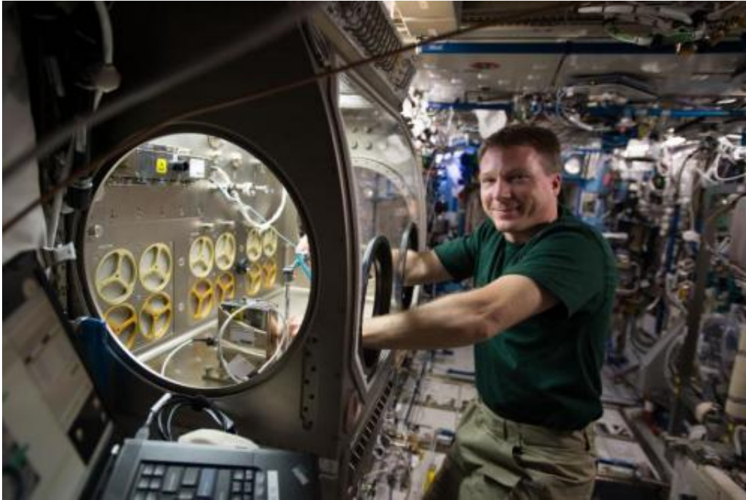
Expedition 42 Flight Engineer Terry Virts sets up the Microgravity Science Glovebox for the Micro-5 experiments. Credit: NASA
