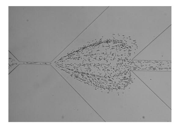
Cells flow at a velocity of 10 cm/s from right to left through the microfluidic channel (width oft the image shown: 1.5 mm). The sheath flow from the upper and lower right corners focuses the cells for cell deformability measurements in the narrowest part of the channel. Credit: Image: project ZellMechanik Dresden
