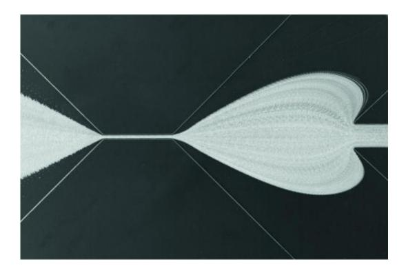
Cells flow at a velocity of 10 cm/s from right to left through the microfluidic channel (width of the image shown: 1.5 mm). The sheath flow from the upper and lower right corners focuses the cells for cell deformability measurements in the narrowest part of the channel. This focusing causes the formation of heart-shaped streamlines as illustrated here by an inverted overlay of many single frames. Credit: ZellMechanik Dresden
