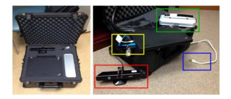
The Lab-in-a-Box complete data collection infrastructure can be easily transported on site and set up in minutes, including sensing and recording components that need to be set up for data collection. Highlighted in red is the Microsoft Kinect sensor; in green, the SMI eye tracker; in yellow, the cables connecting to the Epiphan frame grabber and to the physician's workstation; and in blue, the main power outlet to power up the Lab-in-a-Box. Credit: UC San Diego/VA
