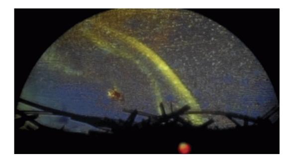
The engineers found relatively large fragments could ignite blazes even at low temperatures, if the fuel was of a certain type. Large shards might come from overheated vehicle brakes, bearings or result from sloppy welding. Credit: James Linwood Urban, Combustion and Fire Processes Laboratory, University of California - Berkeley
