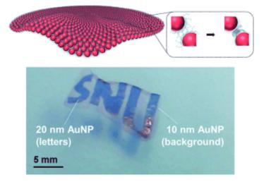
Free-standing nanoparticle films are of great interest for technical applications, such as the development of nanoelectronic devices. In the journal *Angewandte Chemie*, Korean scientists have introduced very flexible and stable monolayers of gold nanoparticles made by a self-assembly process based on protein aggregation. The films were used to coat wafers up to 10 cm in diameter.
