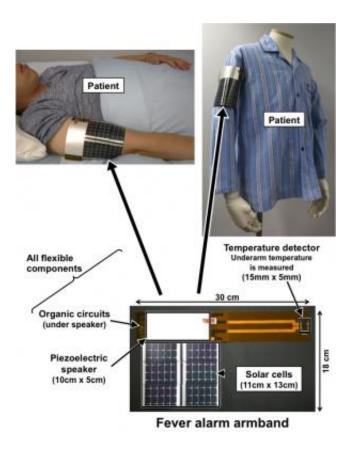
The armband is 30 cm long and 18 cm wide, and can be worn either directly on the skin or on top of clothing. The device is designed so that the thermal sensor is located between the arm and the body. The organic power supply circuit is located under the piezo film speaker to reduce surface area. Credit: © 2015 Sakurai Lab. / Someya Lab.
