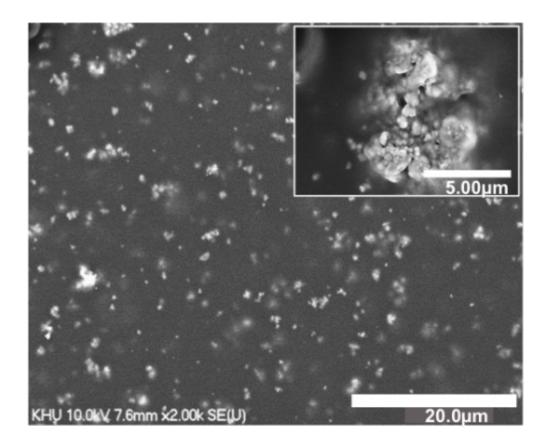
This electron microscope image shows tiny nanoparticles of bismuth ferrite embedded in a polymer film. The film enhances the unique electric and magnetic properties of bismuth ferrite and preserves these properties even when bent. Credit: YoungPak Lee/ Hanyang University
