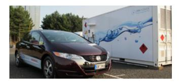
ITM Power's hydrogen refuelling station, HFuel, generates hydrogen by electrolysis
